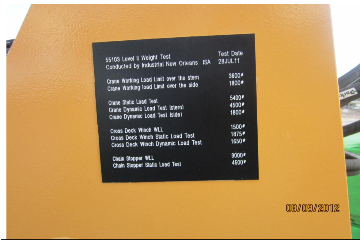
Photo 12, Deck crane weight test results.
