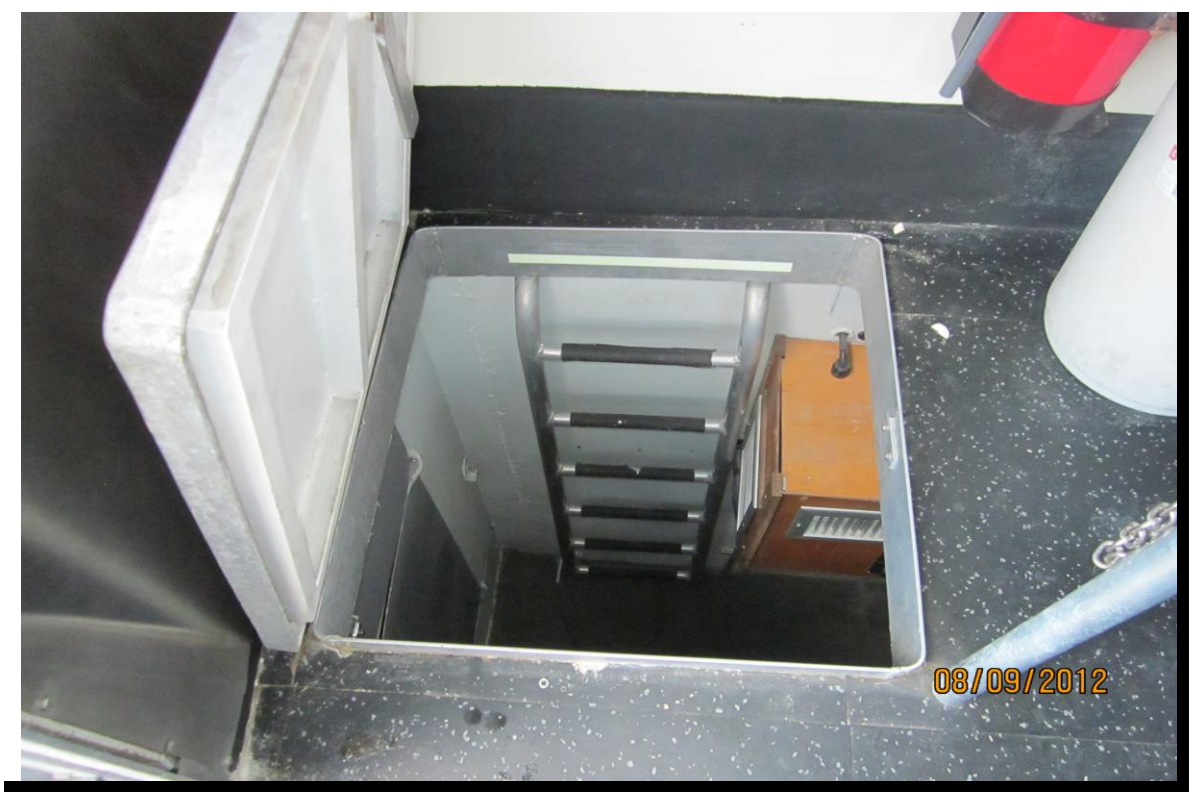
Photo 7, Hatch from pilot house to sleeping quarters.
