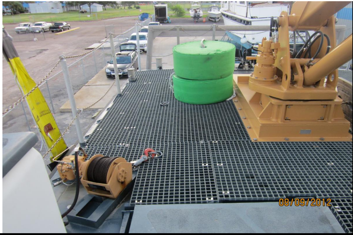
Photo 10, Stbd. aft deck. Note safety grating on deck.
